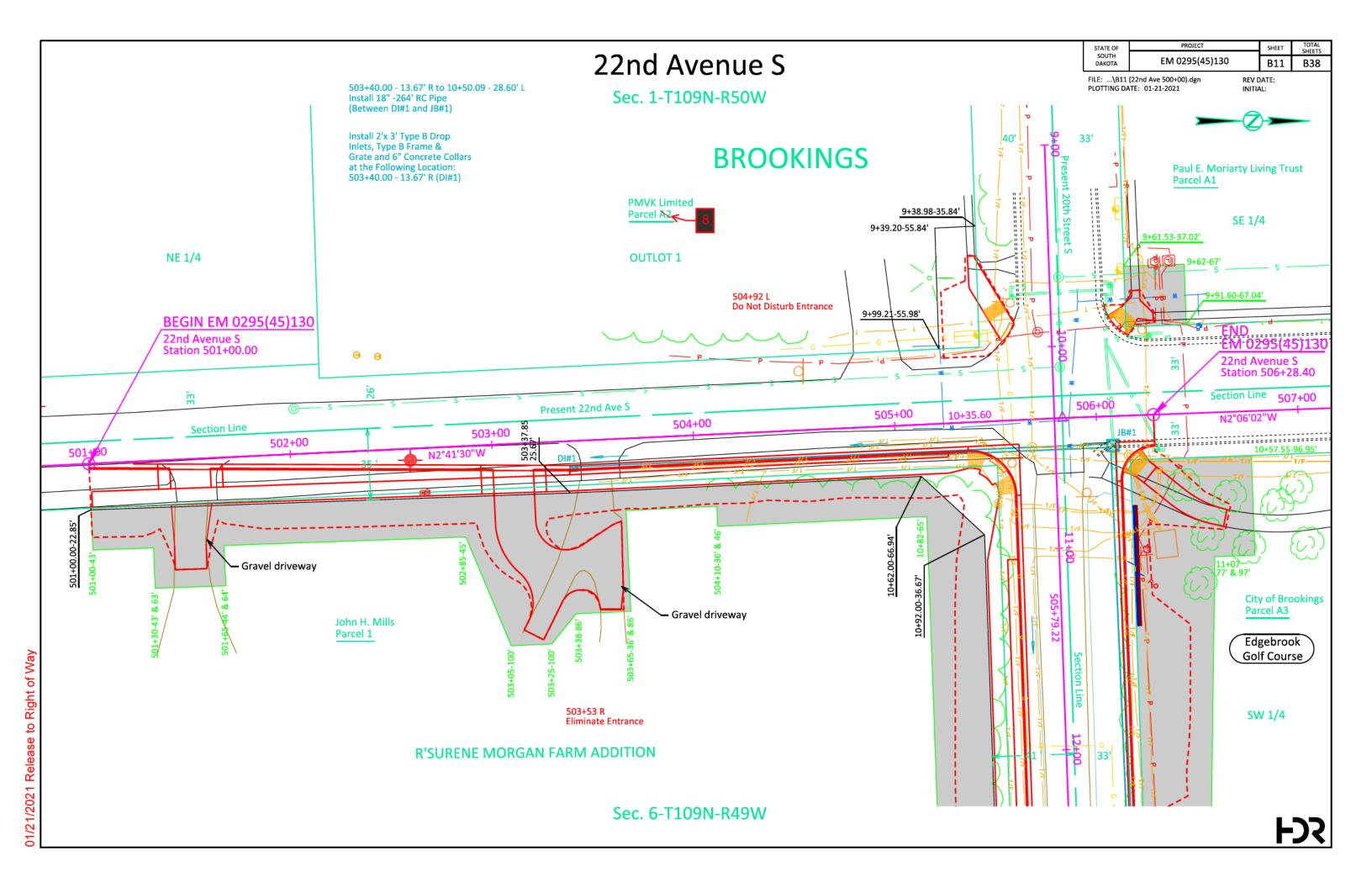
STATE OF SOUTH DAKOTA 22nd Avenue S Profile EM 0295(45)130 B12 FILE: ...\B12 (22nd Ave 500+00)P.dgn PLOTTING DATE: 01-21-2021 REV DATE: INITIAL: 505+79.22 L&R 53' Int Street (20th Street S) 20' Drive 20' Drive DI#1 270'-18" RCP @ 0.56% 01/21/2021 Release to Right of Way 502+00 503+00 504+00 505+00 506+00
