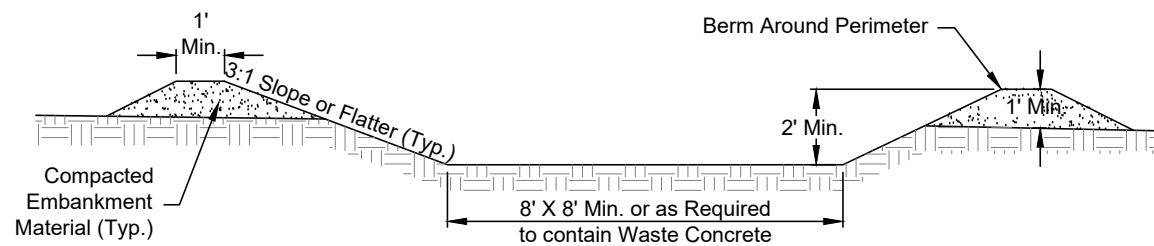
Cross Sectional View Concrete Washout Facility
