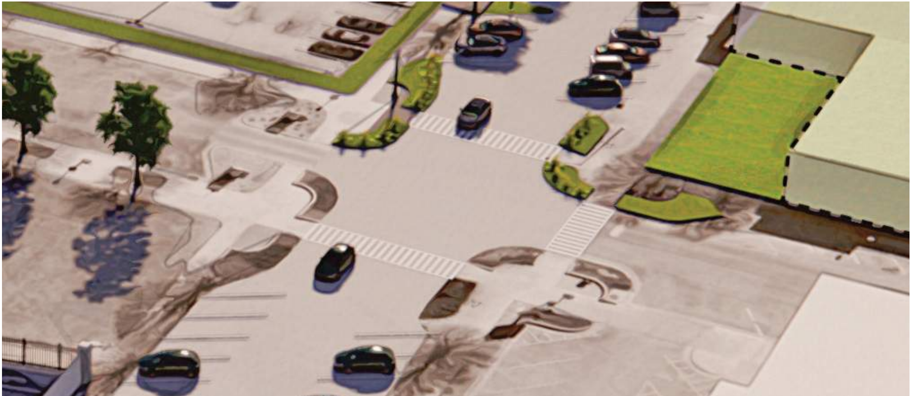
Figure 3.6 — 5th Avenue Bump-out Retrofit
