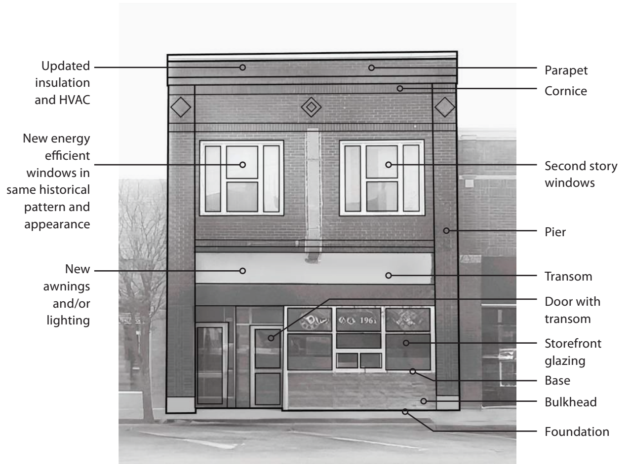
Figure 3.1 — Storefront features and typical improvement opportunities.
