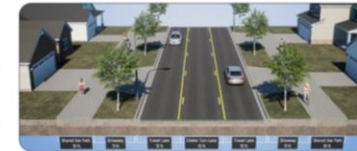
OPTION B: 3-Lane with Two-Way Left Turn Lane and Shared Use Paths
