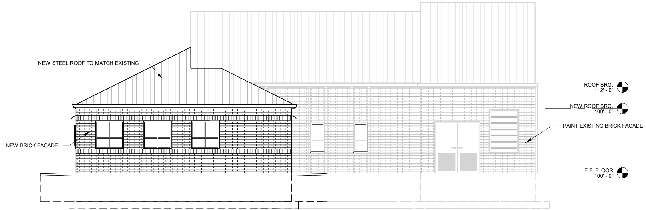
1 EAST ELEVATION A-105 1/8" = 1'-0"
