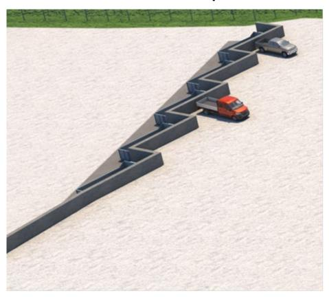
Rendering shows vehicles backed up to wall to dump waste over wall into 30 yrd roll-off containers.
